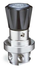
TESCOM 44-2800 Series **tied diaphragm** design provides additional shut-off assistance for toxic or corrosive gases. Positional captured bonnet provides secondary containment for added safety. Available in Hastelloy<sup>®</sup> or Monel materials.
