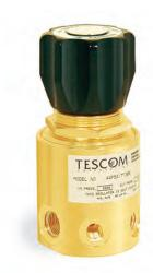
TESCOM 44-1500 Series high flow/low pressure regulator controls outlet pressures up to 600 psig / 41 bar. Large area piston provides accurate pressure control and cycle life superior to diaphragm sensed regulators when applied to heavy duty cycling. Features a segregated/captured vent for hydraulic or pneumatic media and is available in two outlet spring ranges. Optional dome or air loaded versions for remote operation or for use with the TESCOM ER5000 Electropneumatic Controller for automation.
