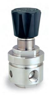
TESCOM 44-3200 Series is a compact, high flow, high purity single-stage regulator for specialty, flammable and industrial gas flows of 5-50 SCFM / 141-1415 SLPM. Diffusion-resistant metal diaphragm seal ensures gas purity and integrity.
