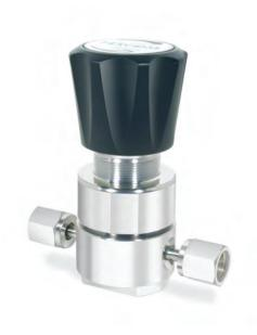
TESCOM 22-2200 Series high purity BA Grade pressure reducing regulator provides 316 Stainless Steel construction with 25 R<sub>a</sub> surface finish and is electronic grade cleaned. Inlet pressure is 250 psig / 17.2 bar with outlet pressures up to 150 psig / 10.3 bar.
