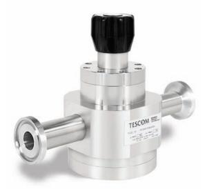
TESCOM PH-1800 Series is part of our Pharmpure<sup>™</sup> product line. This high purity, high-flow singlestage regulator offers a compact, USP Class VI and BPE compliant design suitable for biotech and pharmaceutical applications. This regulator offers gas flows of 5-2000 SCFM /142-56,634 SLPM. Its Gylon<sup>®</sup> diaphragm ensures gas purity and integrity.
